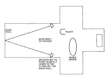
Fig. 8 The working layout of the speakers in the church.
