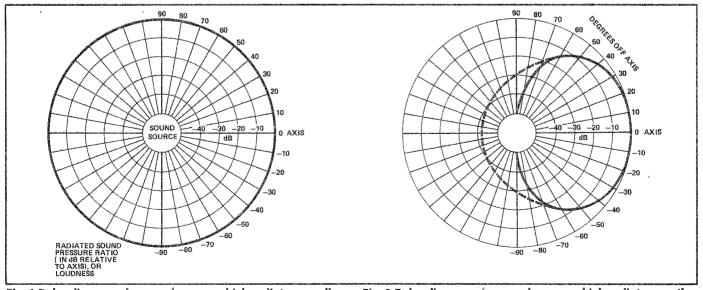
Fig. 1 Polar diagram of a sound source which radiates equally in all directions (approximated by an unmounted loudspeaker). The sound source is at the centre of the diagram.
