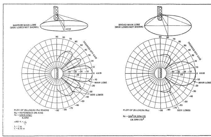
Fig. 3 Polar diagram of a column loudspeaker at 1 kHz.
