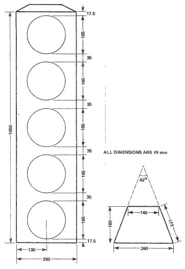
Fig. 7 Cabinet details — all dimensions are in millimetres. The total cabinet volume is 0.324 cubic metres. A suitable material to use is  $\frac{34}{7}$  chipboard and this thickness needs to be added to the dimensions shown where appropriate.
