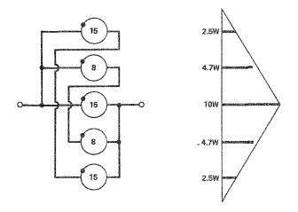
Fig. 5 The wiring diagram for the 8 and 15 ohm speakers. Note how each speaker is wired in phase. For 10 W speaker units the power handling is about 25 W (actually 24.375 W). At right is shown the profile of the graded aperture.
